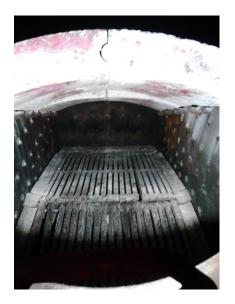
The last fire brick has been fitted into place — it caused more trouble than all of the others combined, as it had to be removed and trimmed three times before it slotted into place properly. Geoff was quite pleased to see it finally in place!
