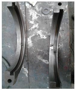
While working on the brake calipers, it was found that an axle suspension bearing dust guard had a broken locating pin, so Joe has made a replacement pin.
